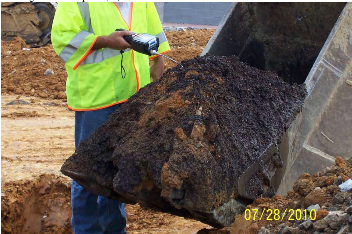
View of soil scanning and PID used during removal of impacted soil.
